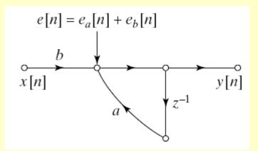
Zero-Input Limit Cycles in Fixed-Point Realization of IIR Filters
