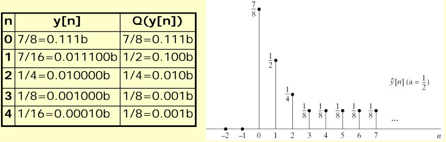
• A finite input caused an oscilation with period 1
